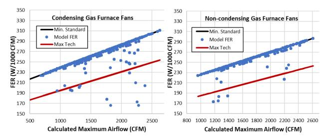
**Figure 1:** Furnace fan FER (W/1000 CFM) vs. calculated maximum airflow for condensing (left) and noncondensing (right) non-weatherized gas furnace fans. Black and red lines represent the current minimum standard and the max-tech level from the previous rulemaking analysis, respectively.
